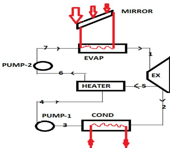
Figure: 3 Model for organic Rankine cycle with regeneration
